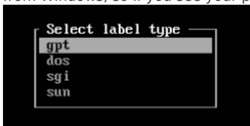
Here, choose `gpt` (GUID Partition Table) for drives bigger than 2 TB and machines using UEFI and `dos` (Master Boot Record) otherwise. Once you come to this screen, you can skip the next step.
